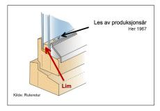
PCB: Norwegian-produced 1965-1975, foreign up to and including 1979. Windows containing chlorinated paraffins: Norwegian-produced from 1976 up to an including 1990, foreign from 1980 up and to 1990.
